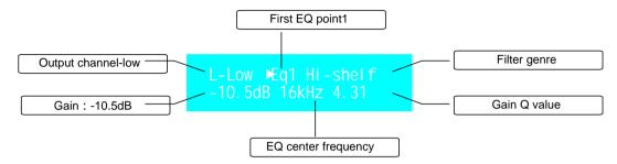
Press the channel choose key and choose the related channel need to be adjusted and press the Para key to choose the parameter which can be changed by the key of +/--.
